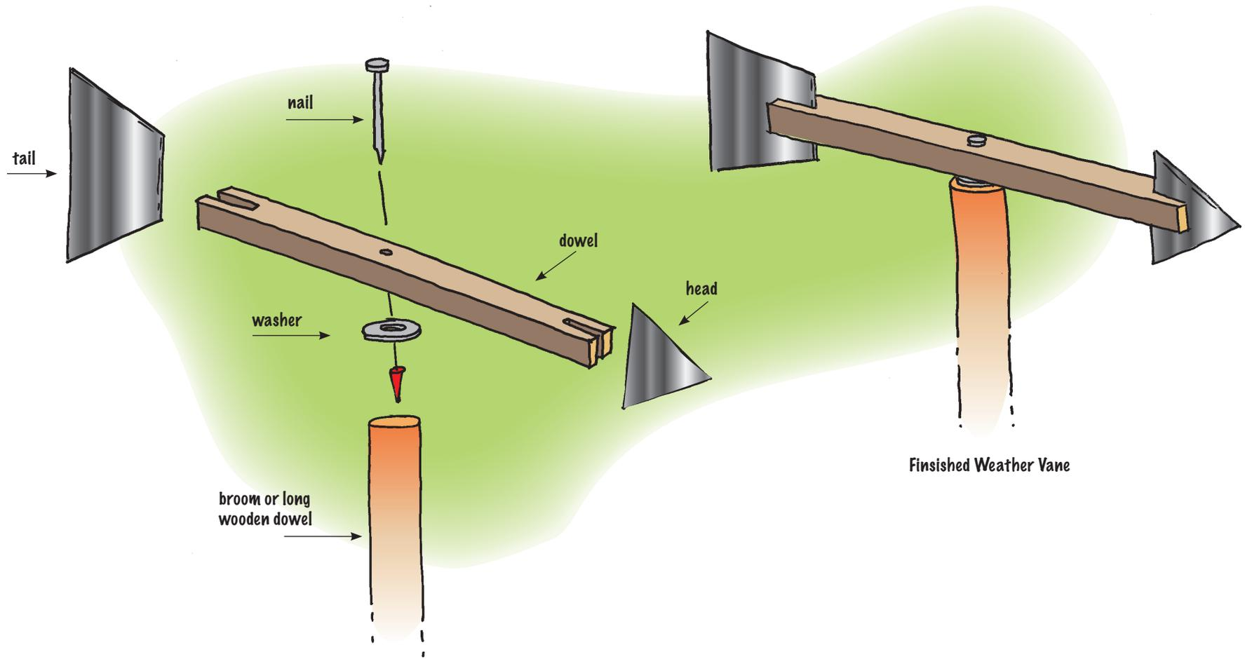
4. Fit the head piece into one of the slots in the wood stick and fit the tail piece into the other slot. Glue the head and tail pieces into place and allow the glue to dry.
